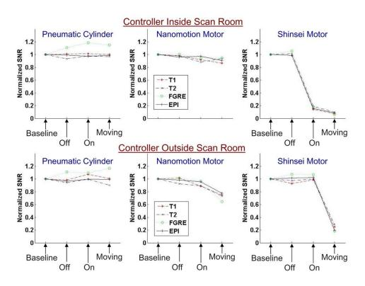
Figure 2.1.1 - Signal-to-Noise ratio using ultrasonic motors<sup>[3]</sup>
