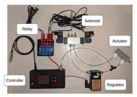
Air from the regulator flows to both the controller and actuator using the T-connector.
