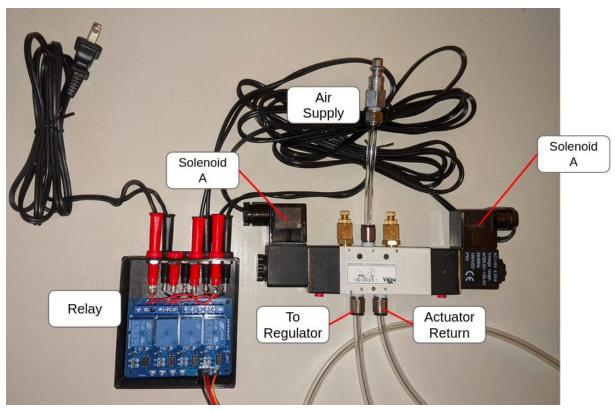
Figure 3.1.1 - Solenoid diagram
